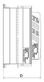
Control voltage (terminal A1, A2) = 230AC D = 302 Digital control voltage (terminal 1-5) = 24DC H = 691 Kg = 42.2 W = 480
